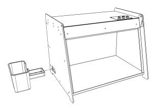
Open the chamber door, slide the fan bracket up, and place one (1) humidity filter inside the water tray. Lower the fan bracket over the filter.
