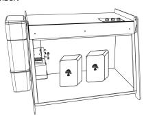
Slide the water tray into the unit through the opening on the left-side wall.
